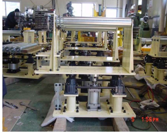
DIVERTER (WEIGHT:600Kg) IP900F TYPE
