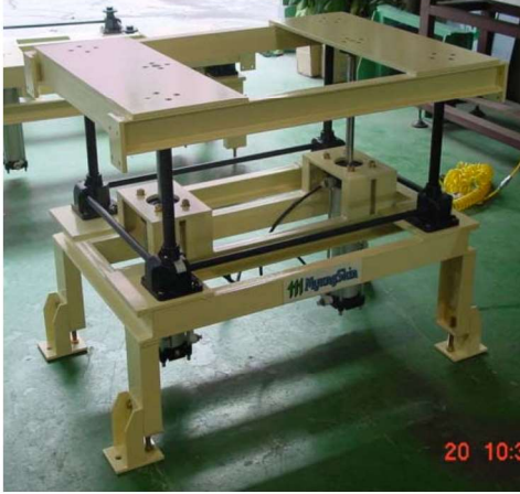
UP/DOWN LIFTER (WEIGHT: 1000Kg) IP1500F TYPE
